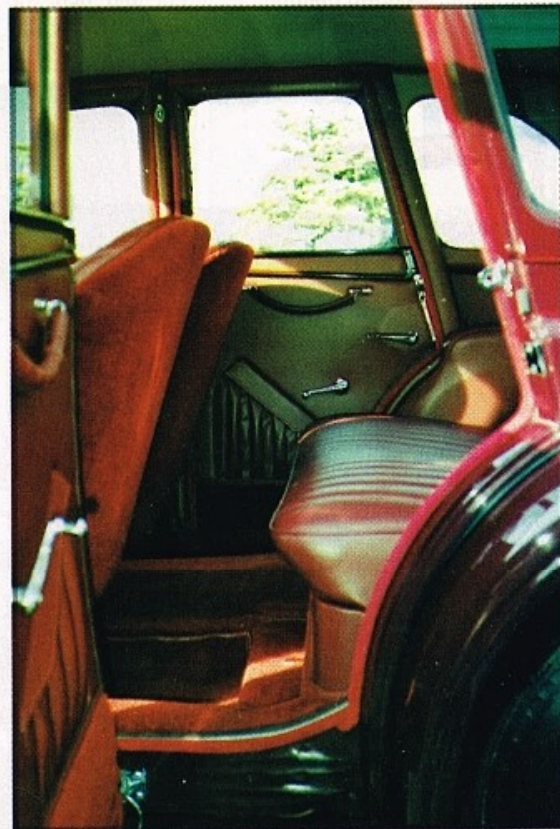
Bernice and Jim combined their skills to re-upholster the car themselves in Australian-sourced vinyl
